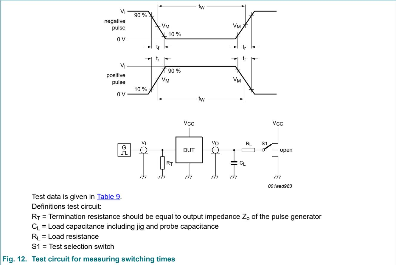
Fig. 12. Test circuit for measuring switching times
