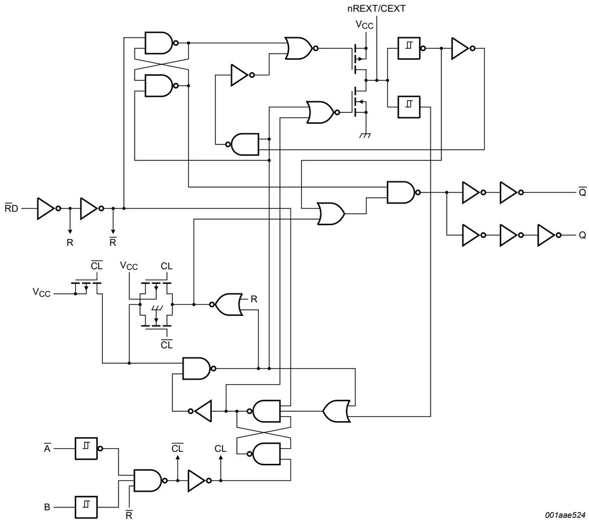
For minimum noise generation it is recommended to ground pins 6 (2CEXT) and 14 (1CEXT) externally to pin 8 (GND).
