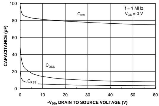
Figure 8. Capacitance Characteristics.
