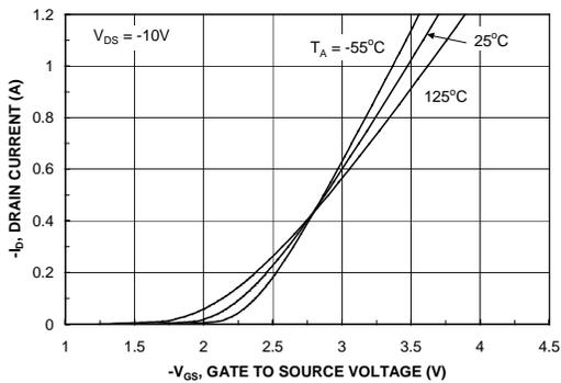
Figure 5. Transfer Characteristics.
