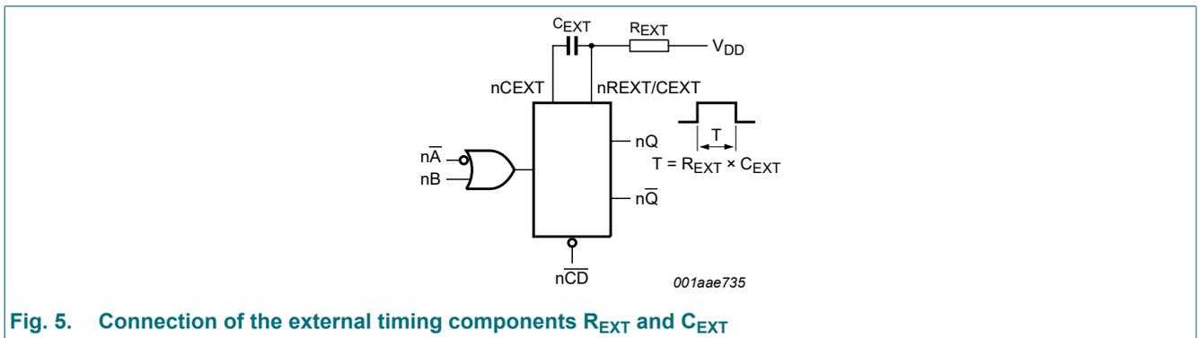
Fig. 5. Connection of the external timing components  $R_{EXT}$  and  $C_{EXT}$
