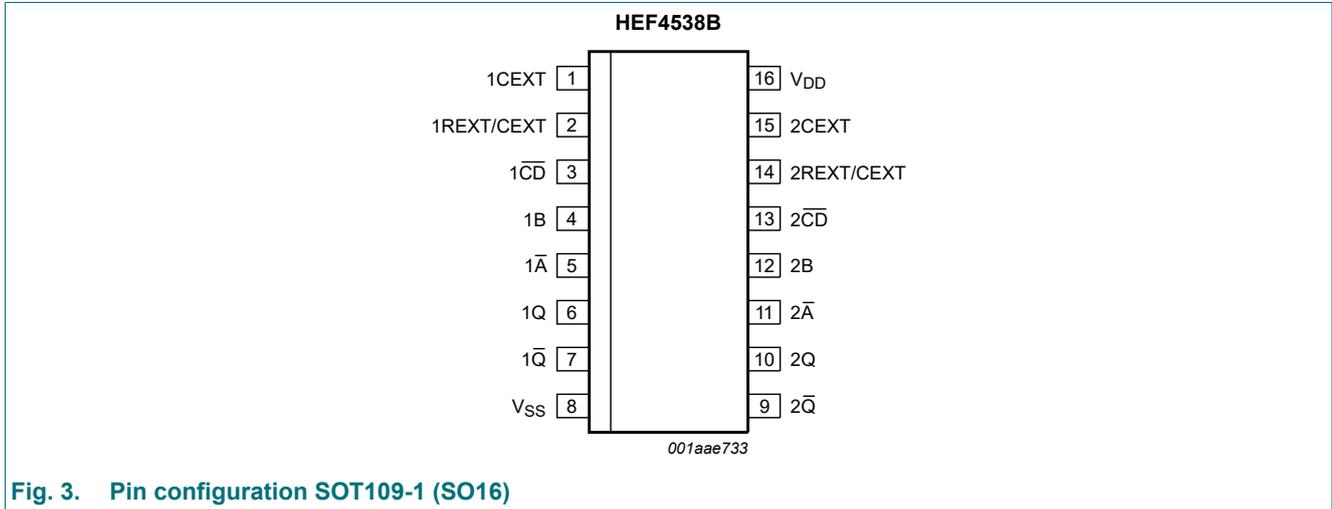
Fig. 3. Pin configuration SOT109-1 (SO16)
