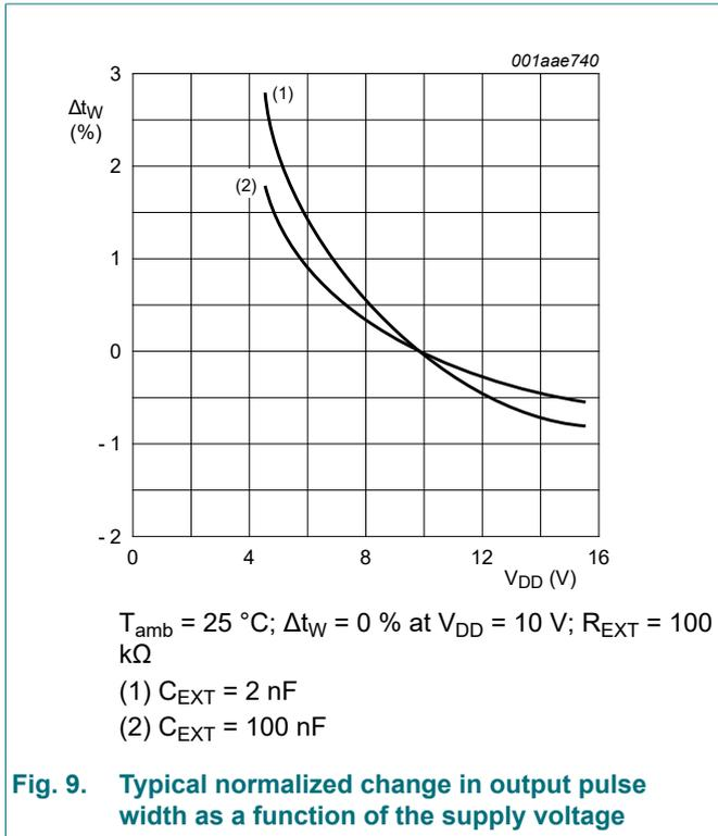
Fig. 9. Typical normalized change in output pulse width as a function of the supply voltage
