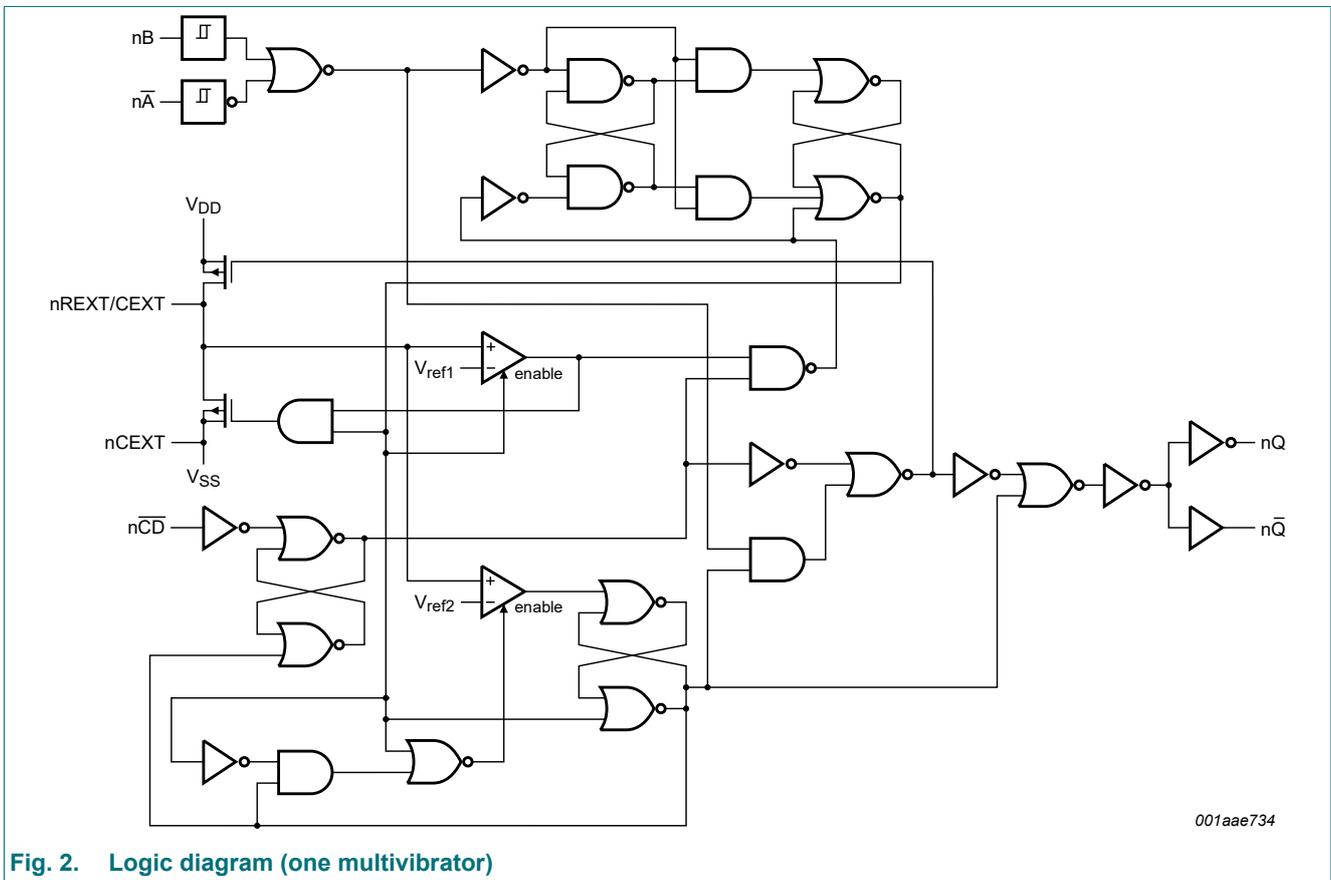
Fig. 2. Logic diagram (one multivibrator)
