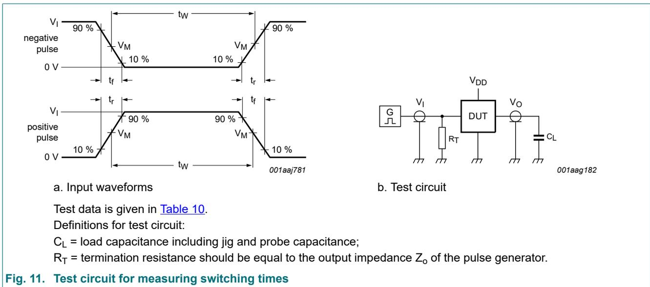
Fig. 11. Test circuit for measuring switching times
