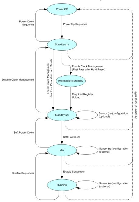
Figure 12. VITA 25K Sensor Operation Flow
