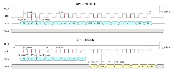
Figure 17. SPI Read and Write Timing Diagram
