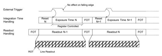
Figure 10. Triggered Shutter Operated in Master Mode
