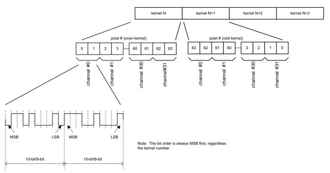
Figure 33. Data Output Order when Subsampling is Disabled
