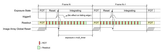
Figure 20. Exposure Time Control in Triggered Global Mode (Master)
