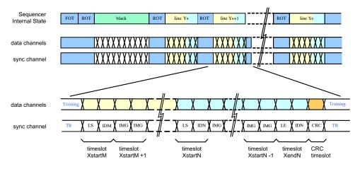
Figure 30. Timeline Showing Readout of Two Overlapping Windows
