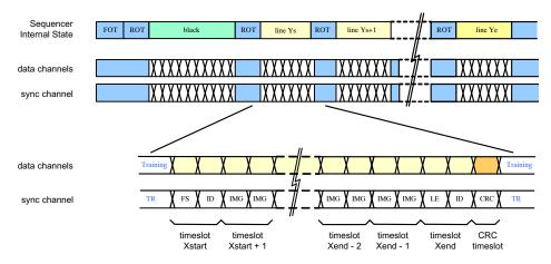
Figure 29. Timeline for Single Window Readout
