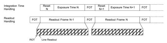
Figure 8. Integration and Readout for Pipelined Shutter
