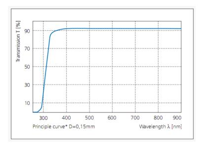
Figure 39. Transmission Characteristics of Glass Lid
