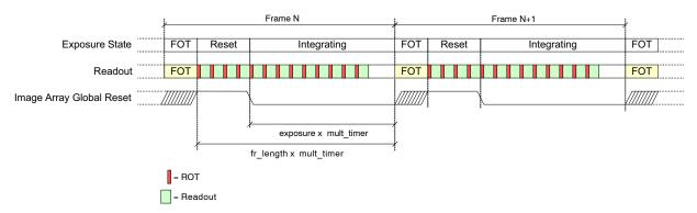
Figure 19. Integration Control for Pipelined Global Shutter Mode (Master, fr mode = 0x1)
