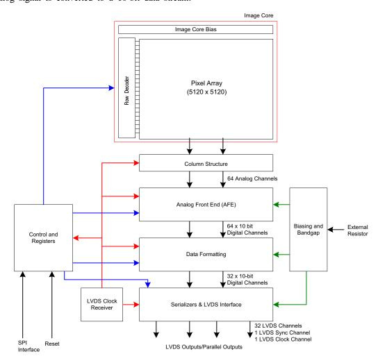
Figure 5. Block Diagram
