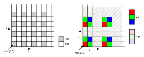
Figure 26. Subsampling Scheme for VITA 25K
