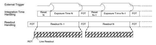
Figure 9. Pipelined Shutter Operated in Slave Mode
