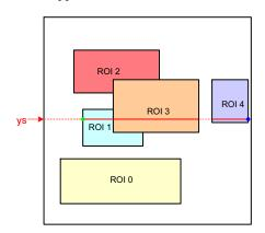
Figure 25. Scanning the Image Array with Five Subwindows
