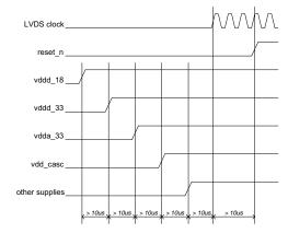
Figure 13. Power-up Procedure
