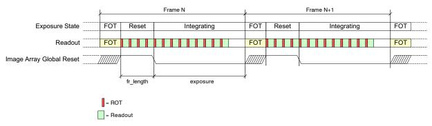
Figure 18. Integration Control for Pipelined Global Shutter Mode (Master, fr mode = 0x0)
