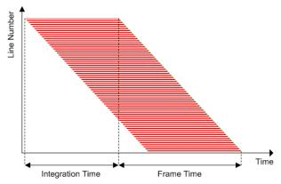
Figure 11. Rolling Shutter Operation
