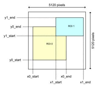
Figure 24. Overlapping Multiple Window Configuration
