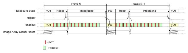
Figure 21. Exposure Time Control in Global-Slave Mode
