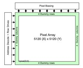
Figure 6. Image Core Diagram
