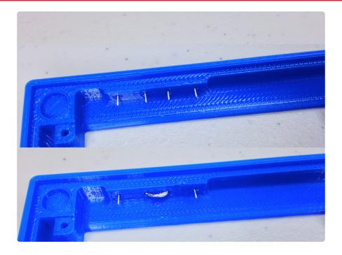
On the inside, you should be able to see all four pins of the pushbuttons. Bend the inner two and join them together with some solder.
