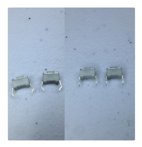
Use a pair of pliers to straighten the legs of the two pushbuttons and then insert them into the cavities on the left side of the enclosure.
