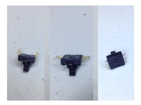
To prepare the joystick for soldering/mounting, straighten its legs, bend them 90 degrees outward, and then cut them to about half the length.
