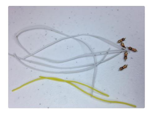
Prepare 5 pairs of resistors and short wires (about 8cm each). We'll cut them to the exact lengths needed later.
