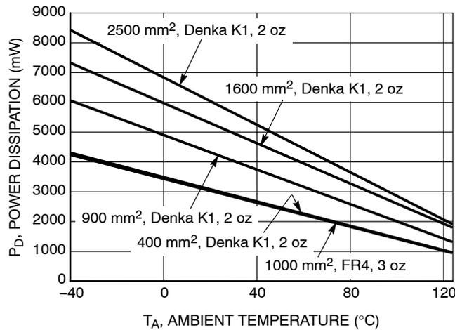
**Figure 6. Power Dissipation vs. Ambient Temperature @  $T_J = 175^\circ\text{C}$**
