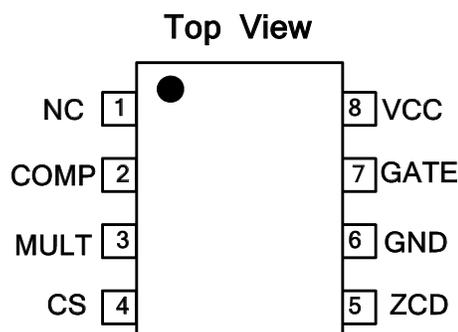
Figure 2: Pin Assignments
