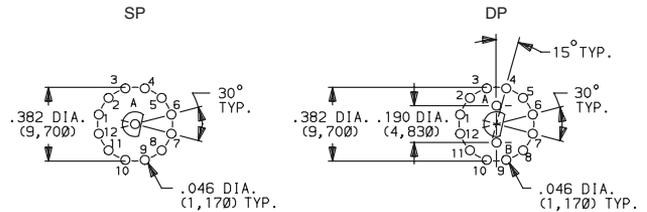
Actuators and schematics shown in pos. 1.
