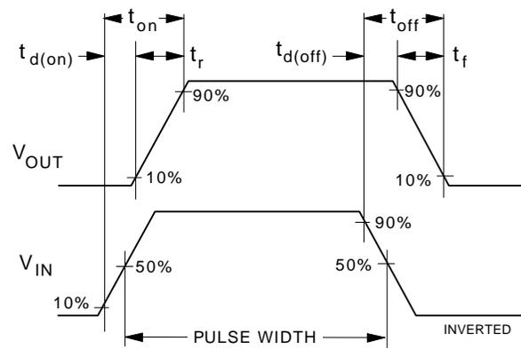
Figure 12. Switching Waveforms.
