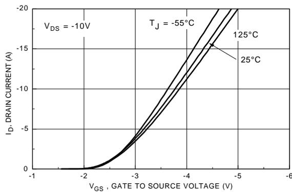
Figure 5. Transfer Characteristics.
