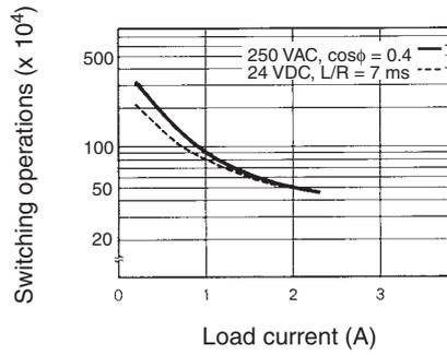
Reference: A maximum current of 0.6 A can be switched at 125 VDC (cosφ = 1).
