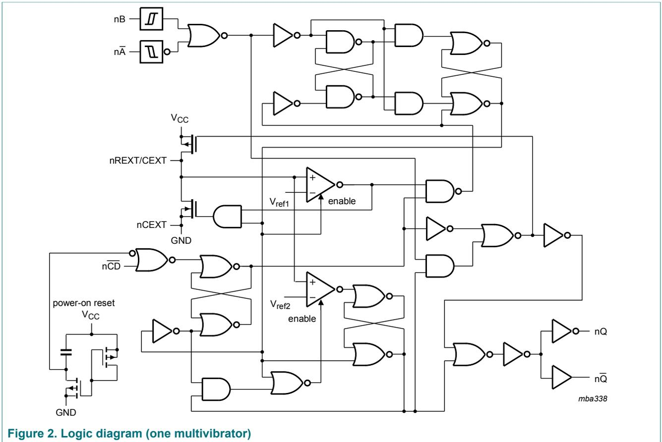
Figure 2. Logic diagram (one multivibrator)
