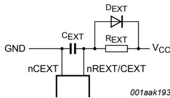
Figure 10. Power-down protection circuit
