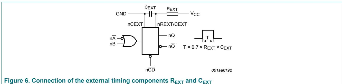
Figure 6. Connection of the external timing components R<sub>EXT</sub> and C<sub>EXT</sub>
