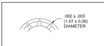
External shorting links, as shown in the drawing, can be used in place of conventional solder lug terminals in the Series 5000, 24, 42 or 43 rotary switches. Shorted terminals can also be accomplished internally in the Series 71 rotary switches. Solder lug terminals can be intermixed on the same deck.
