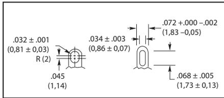
Series 08A, 09A, 42H, 42M, 44H, and 44M: Lug terminals for several wires; standard in Series 08M, 09M, 53, 57, and 59 switches.
