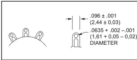
The gold-plated terminal features a slot to accept wires in addition to the conventional wire hole.
