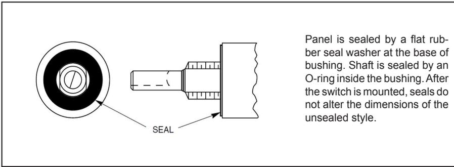
Panel is sealed by a flat rubber seal washer at the base of bushing. Shaft is sealed by an O-ring inside the bushing. After the switch is mounted, seals do not alter the dimensions of the unsealed style.
