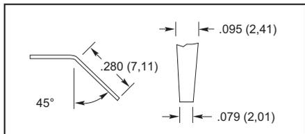
Used in place of conventional solder lug terminals. Taper tab terminals are gold plated.
