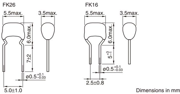
**RATED VOLTAGE E<sub>dc</sub>: 100 to 630V**
