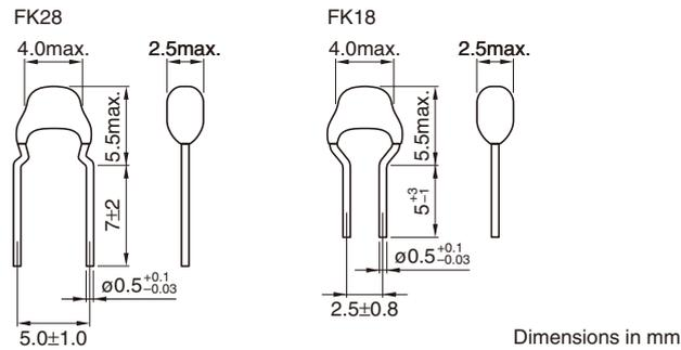
RATED VOLTAGE E<sub>dc</sub>: 100 to 250V
