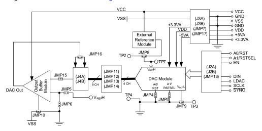
Figure 1. DAC8564/65 EVM Block Diagram
