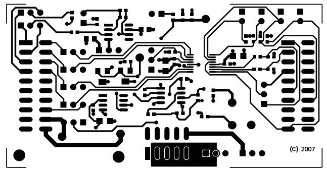
Figure 3. Layer 1 (Top Signal Plane)
