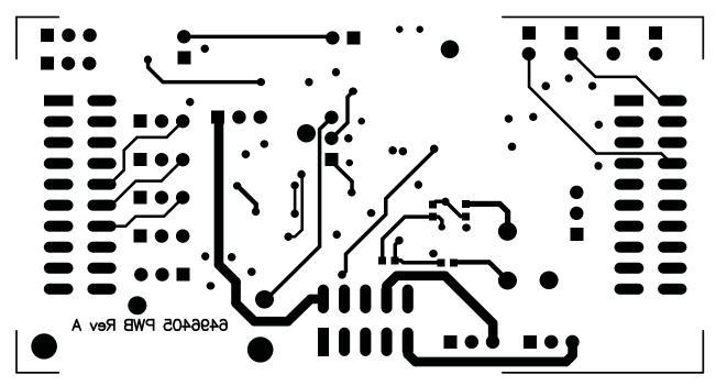
Figure 6. Layer 4 (Bottom Signal Plane)
