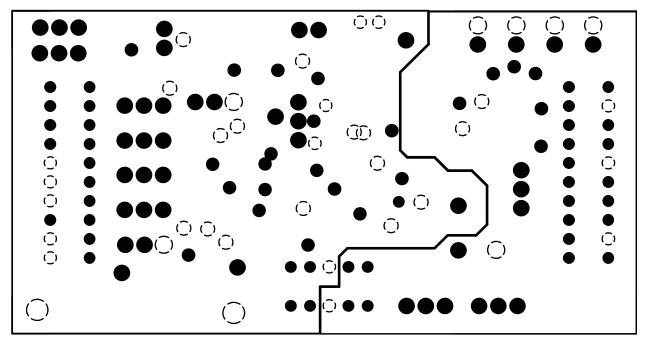
Figure 4. Layer 2 (Ground Plane)
