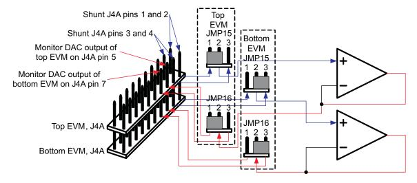
Figure 18. DAC8564/65 EVM Output Operational Amplifier Jumper Configuration for Stacking
