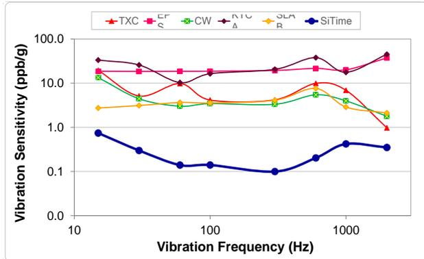
Figure 5. Vibration Robustness<sup>[5]</sup>
