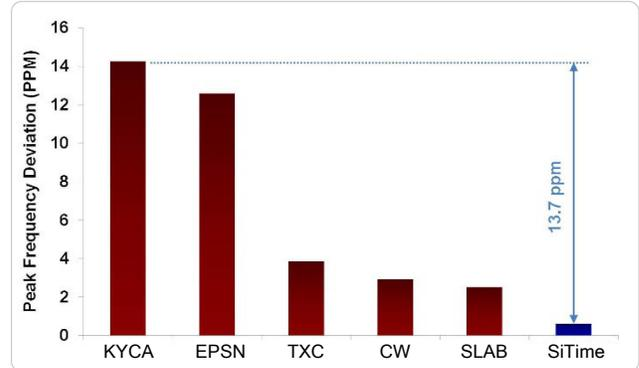
Figure 6. Shock Robustness<sup>[6]</sup>
