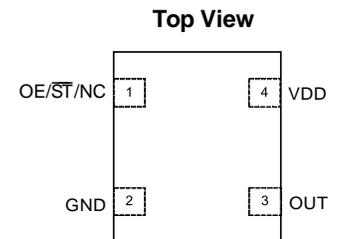
**Figure 1. Pin Assignments**
