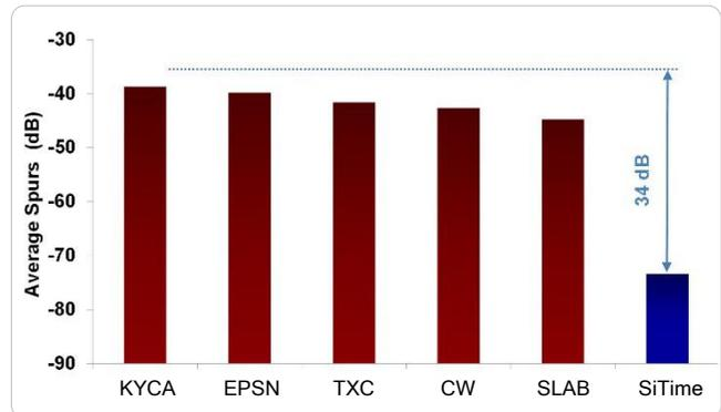
Figure 3. Electro Magnetic Susceptibility (EMS)<sup>[3]</sup>
