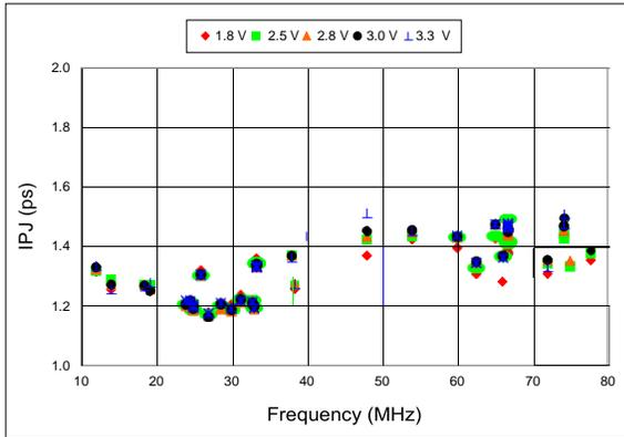
**Figure 14. RMS Integrated Phase Jitter Random (12 kHz to 20 MHz) vs Frequency<sup>[9]</sup>**
