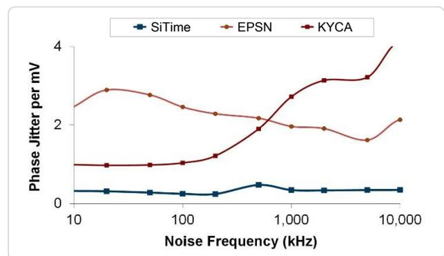
Figure 4. Power Supply Noise Rejection<sup>[4]</sup>
