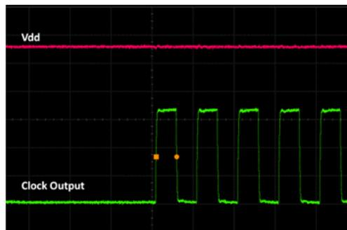
Figure 18. Startup Waveform vs. Vdd
