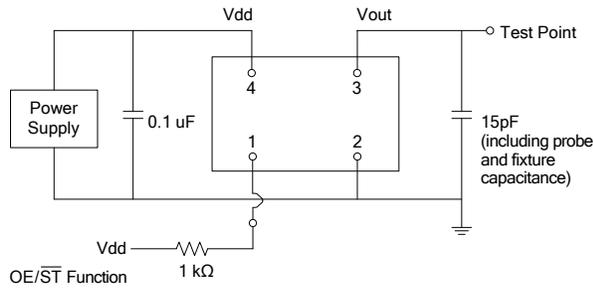
**Figure 2. Test Circuit**
