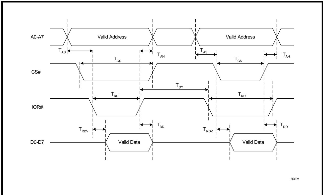
FIGURE 14. 16 MODE (INTEL) DATA BUS WRITE TIMING FOR CHANNELS A-D
