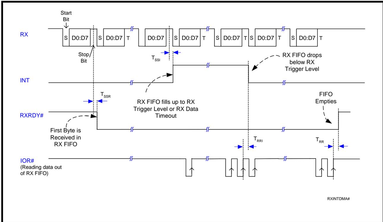
**FIGURE 20. RECEIVE READY & INTERRUPT TIMING [FIFO MODE, DMA ENABLED] FOR CHANNELS A-D**
