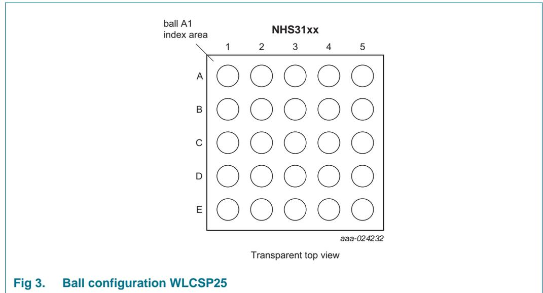
Fig 3. Ball configuration WLCSP25
