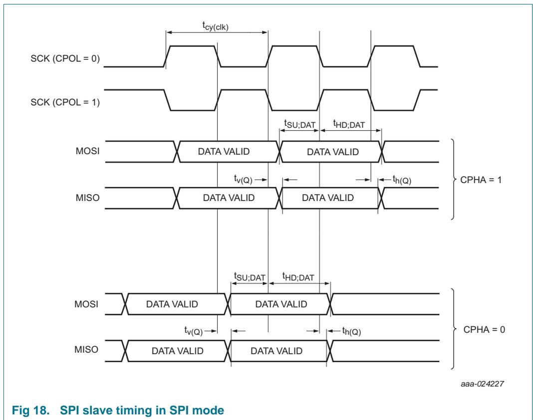
Fig 18. SPI slave timing in SPI mode
