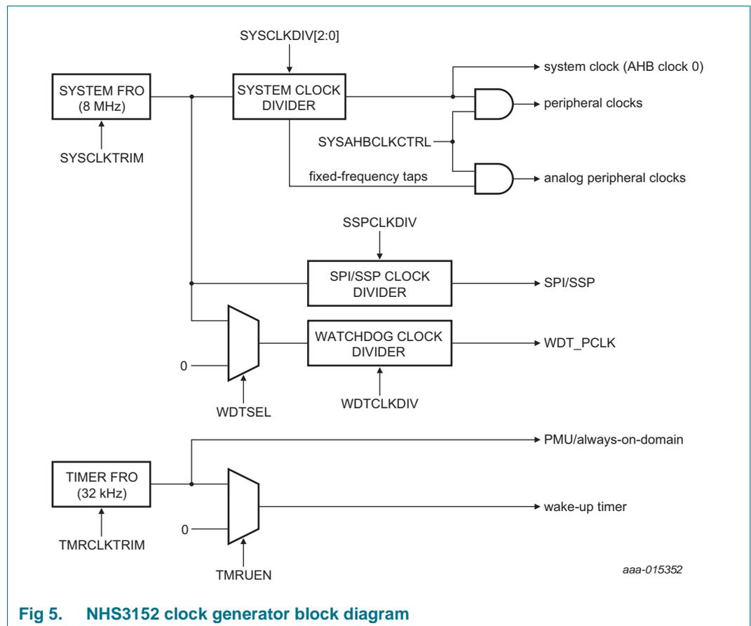
Fig 5. NHS3152 clock generator block diagram
