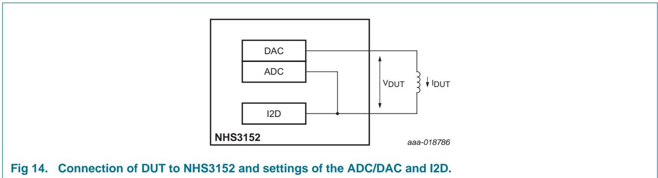
Fig 14. Connection of DUT to NHS3152 and settings of the ADC/DAC and I2D.
