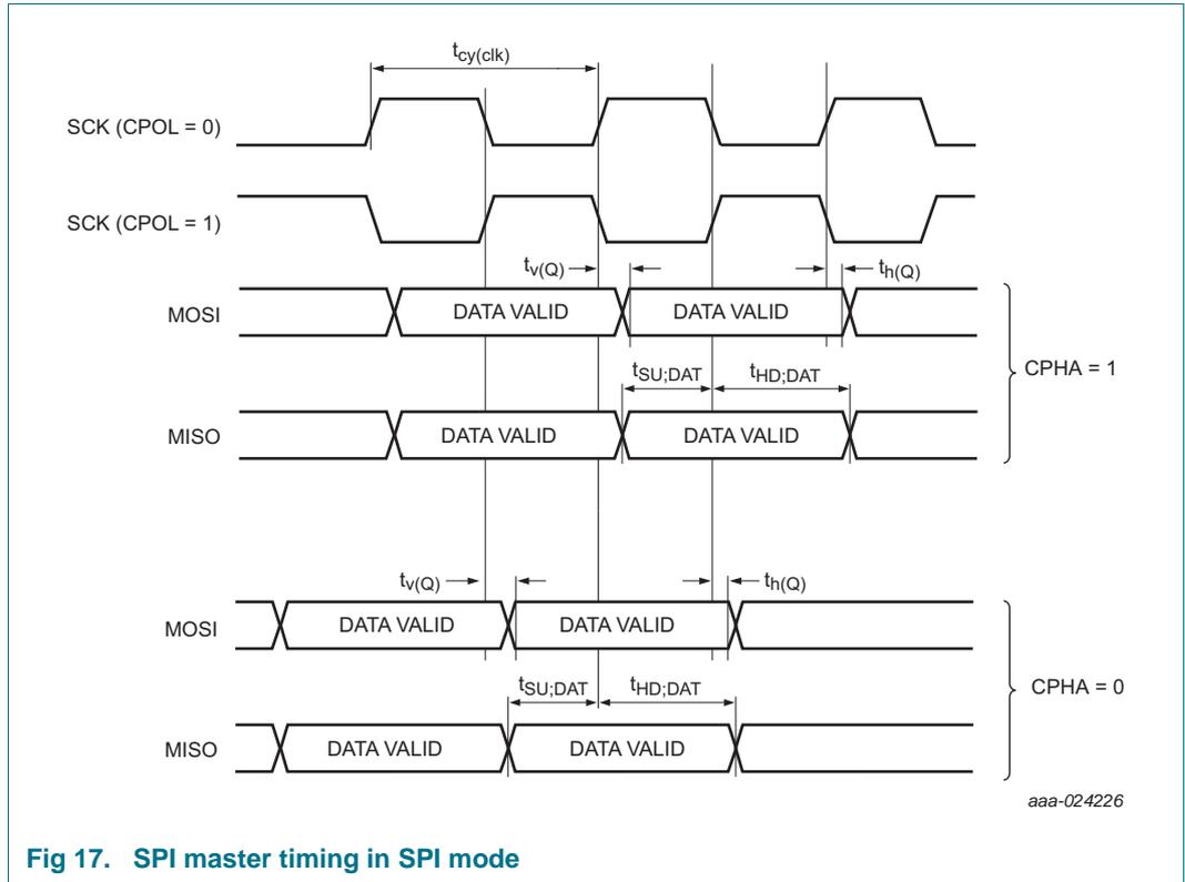
Fig 17. SPI master timing in SPI mode
