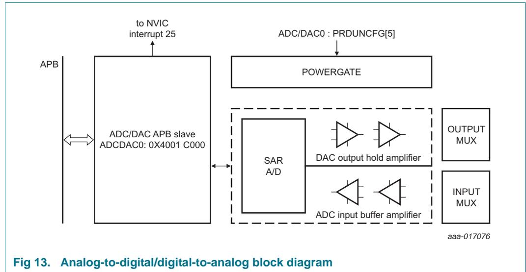
Fig 13. Analog-to-digital/digital-to-analog block diagram
