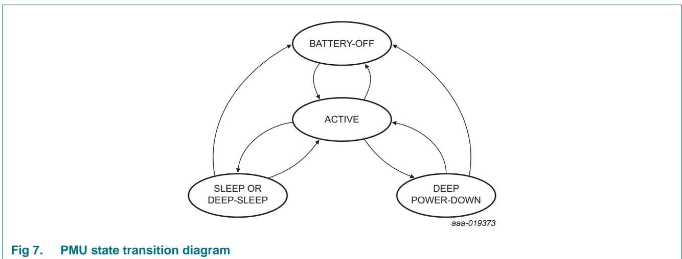
Fig 7. PMU state transition diagram
