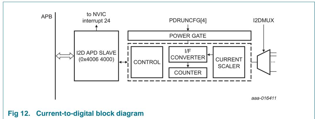
Fig 12. Current-to-digital block diagram
