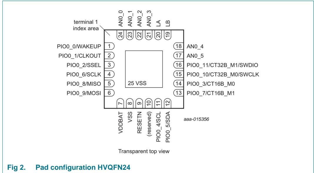
Fig 2. Pad configuration HVQFN24
