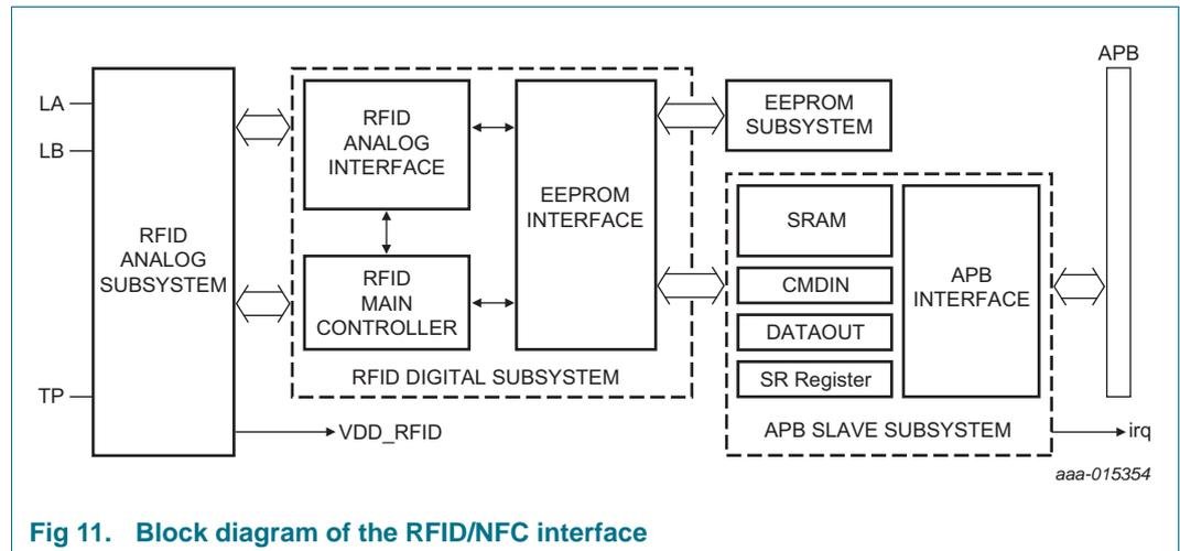
Fig 11. Block diagram of the RFID/NFC interface
