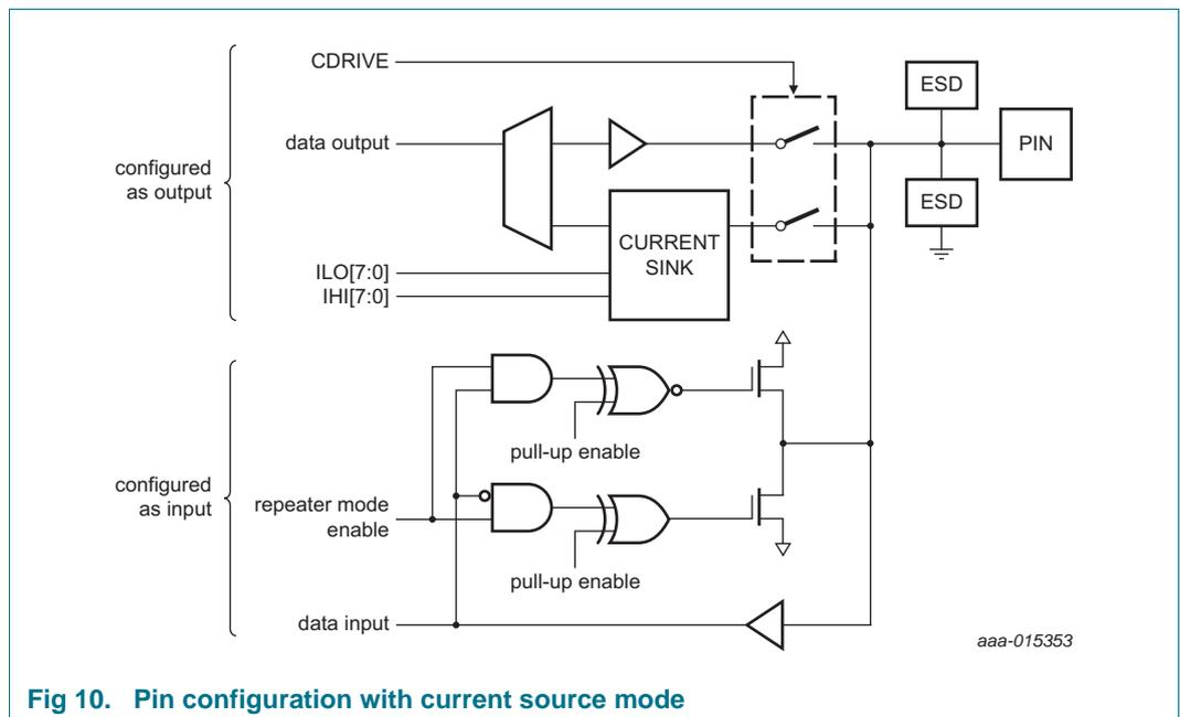
**Fig 10. Pin configuration with current source mode**
