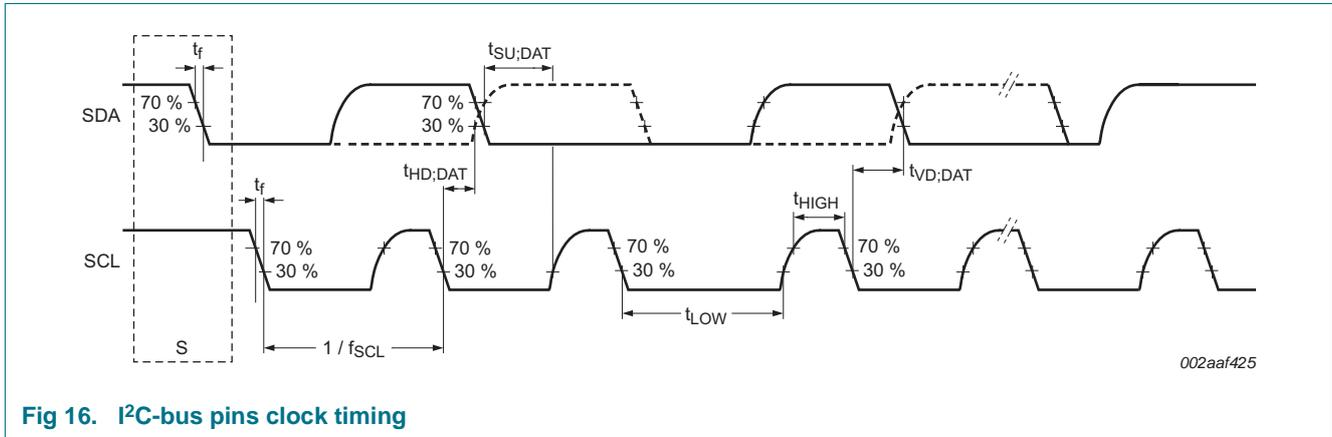
Fig 16. I<sup>2</sup>C-bus pins clock timing
