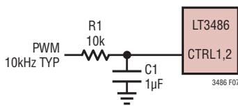
Figure 7. Dimming Control Using a Filtered PWM Signal
