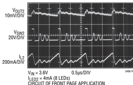
Figure 2. Switching Waveforms
