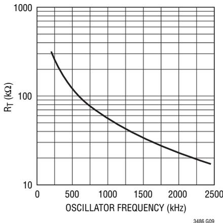
Figure 5. Timing Resistor ( $R_T$ ) Value
