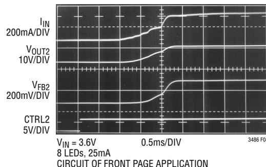
**Figure 4. Start-Up Waveforms**
