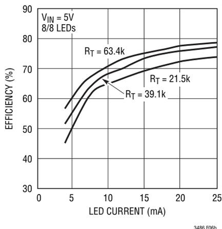
Figure 6b. Efficiency Comparison for Different  $R_T$  Resistors
