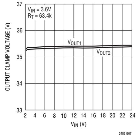
**TYPICAL PERFORMANCE CHARACTERISTICS**  $T_A = 25^\circ\text{C}$  unless otherwise specified.
