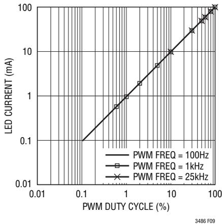
Figure 9. LED Current Variation vs PWM Duty Cycle
