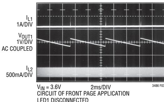
**Figure 3b. Switching Waveforms with Output 1 Open Circuit**
