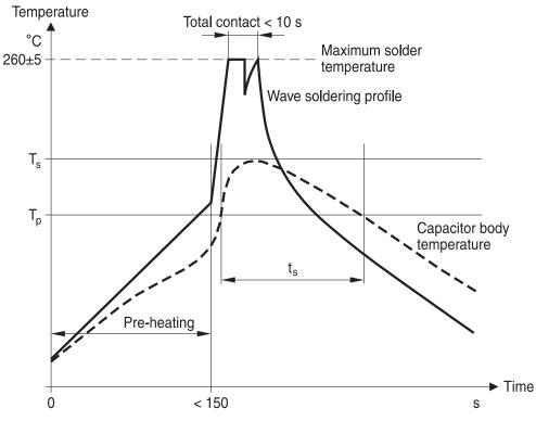
$\label{eq:Ts} T_{s}: \mbox{Capacitor body maximum temperature at wave soldering} $$T_{p}: \mbox{Capacitor body maximum temperature at pre-heating} $$KMK1745-A-E$$
