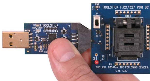
Figure 2. Improper Method of Holding the ToolStick
