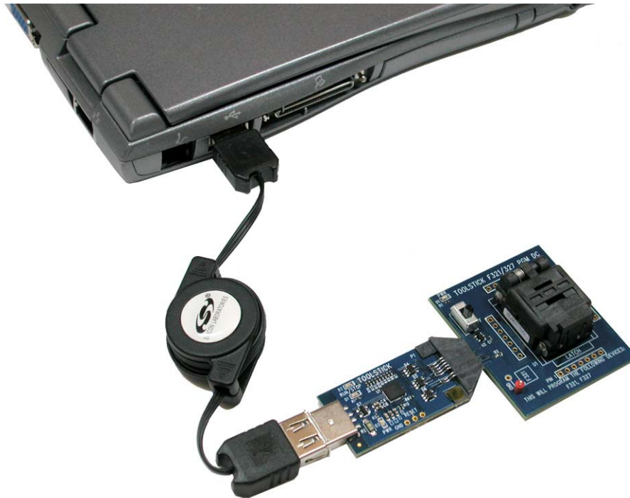
Figure 5. ToolStick Socket Platform Connected to PC
