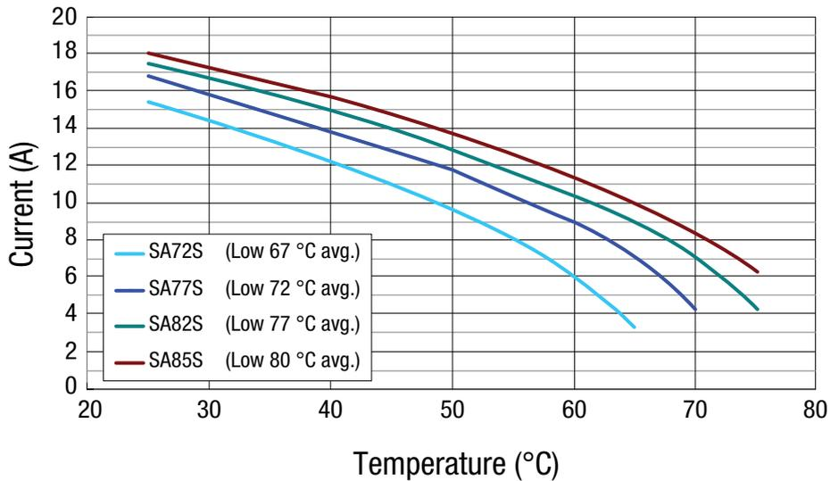
The above curves were derived from placing non-PCB mounted test samples in an oven at 25 °C, 40 °C, 60 °C, and 70 °C, increasing current flow through the sample at a rate of 0.1 A/minute and recording the current value when the sample trips. The current carrying performance is influenced by the PCB design due to copper resistance; users should verify actual device performance in their specific applications.
