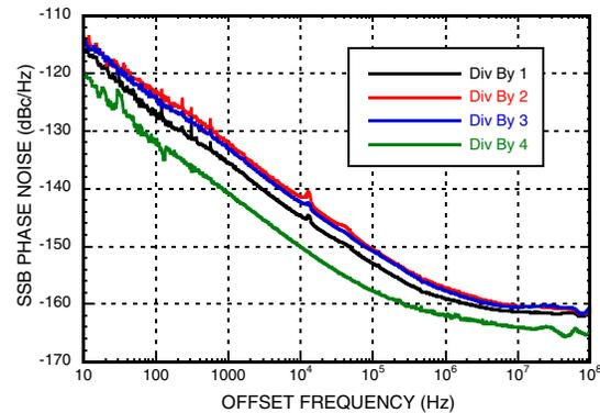
**Phase Noise for 3 Cascaded HMC905LP3E from 6 GHz VCO**
