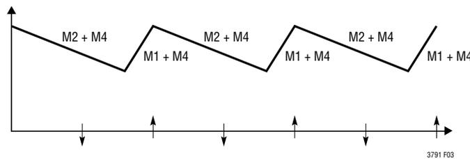
Figure 3. Buck Operation ( $V_{IN} > V_{OUT}$ )
