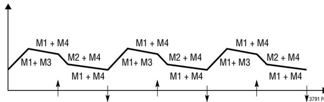
Figure 4. Buck-Boost Operation ( $V_{IN} \leq V_{OUT}$ )
