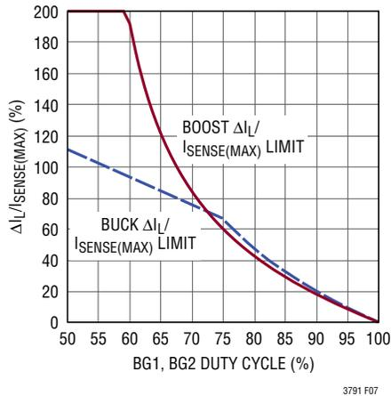
**Figure 7. Maximum Peak-to-Peak Ripple vs Duty Cycle**
