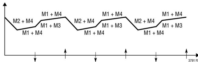
Figure 5. Buck-Boost Operation ( $V_{IN} \geq V_{OUT}$ )
