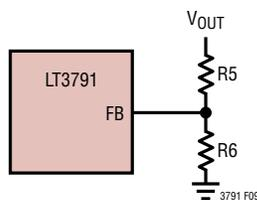
Figure 9. Resistor Connection for Open LED Protection
