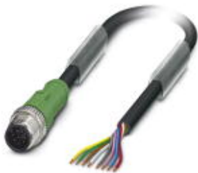
Sensor/Actuator cable, 8-position, PUR halogen-free, black-gray RAL 7021, Plug straight M12, A-coded, on free cable end, Cable length: 3 m
