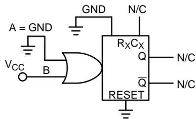
Figure 15. Connection of Unused Section
