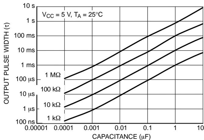
**Figure 3. Output Pulse Width versus Timing Capacitance**
