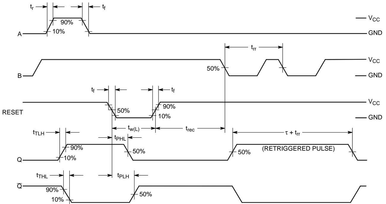
Figure 8. Switching Waveform
