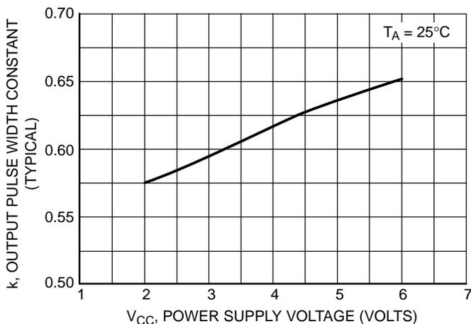
**Figure 2. Typical Output Pulse Width Constant,  $k$ , versus Supply Voltage**
