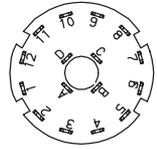
**NOTE:** Switches with 'C' or 'MC' terminations have additional terminal no. 9 as switch support only. This terminal is not connected electrically inside switch. Solder and clean switch base on PC board with other components, then snap on housing/actuator assembly. See page K-7 for installation instructions.
