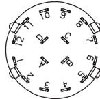
Terminal numbers molded on bottom of housing.
