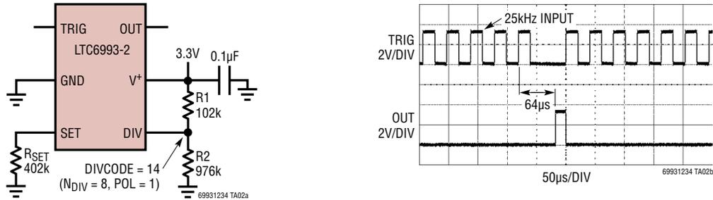
Use retriggerable one shot with output inverted. Output remains low as long as retrigger occurs within  $t_{OUT} = 64\mu s$ .
