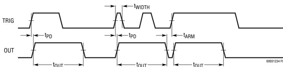
**Figure 3. Non-Retriggering Timing Diagram (LTC6993-1, POL = 0)**
