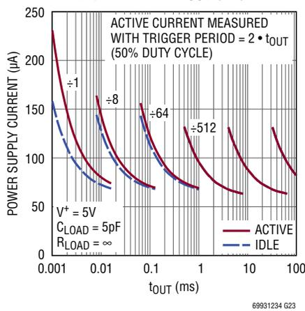
Supply Current vs  $t_{OUT}$  (2.5V)
