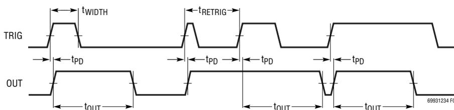
**Figure 4. Retriggering Timing Diagram (LTC6993-2, POL = 0)**
