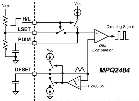
**Figure 7: Two-Step Dimming**
