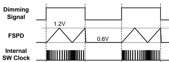
**Figure 10: SW Clock Synchronization by the Dimming Signal**
