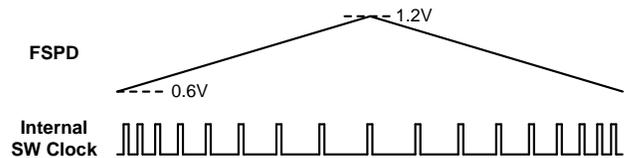
Figure 9: Frequency Spread Spectrum Waveforms
