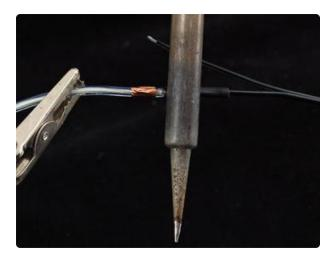
Now you have to heat up the heatshrink to get it to shrink. You can use a heat gun, hair dryer, hold it above a lighter (carefully!) or you can try 'rubbing' the non-solder part of your iron gently against the shrink.
