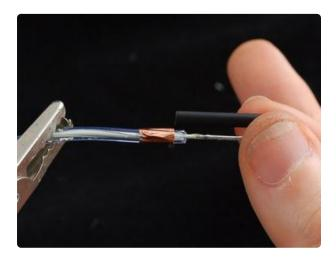
Before you solder it on, get a piece of 1/8" heat shrink and cut it so its as long as the middle wire piece (1/2" or so).
