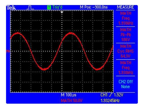
If you are comfortable using tools and want to optimize your driver and wire, you can do so by 'modeling' your EL wire with a capacitor and resistor and plugging that in, then measuring the frequency across the RC with a multimeter or scope, just watch out you don't zap yourself!
