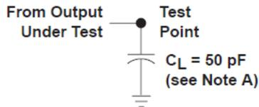
**Figure 7-1. Load Circuit**
