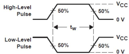
**Figure 7-2. Voltage Waveforms Pulse Durations**
