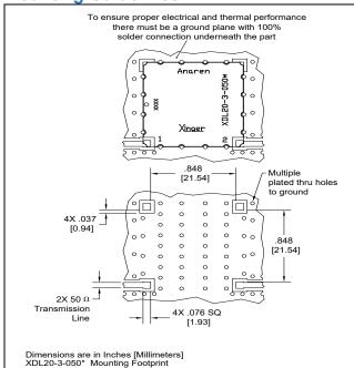
In order for Xinger surface mount delay lines to work optimally, there must be  $50\Omega$  transmission lines leading to and from all of the RF ports. Also, there must be a very good ground plane under the part with a number of plated thru holes to ensure proper electrical performance. If any of these conditions are not satisfied, insertion loss, average delay and VSWR may not meet published specifications
