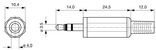
Cable diameter max. 4.0 mm
