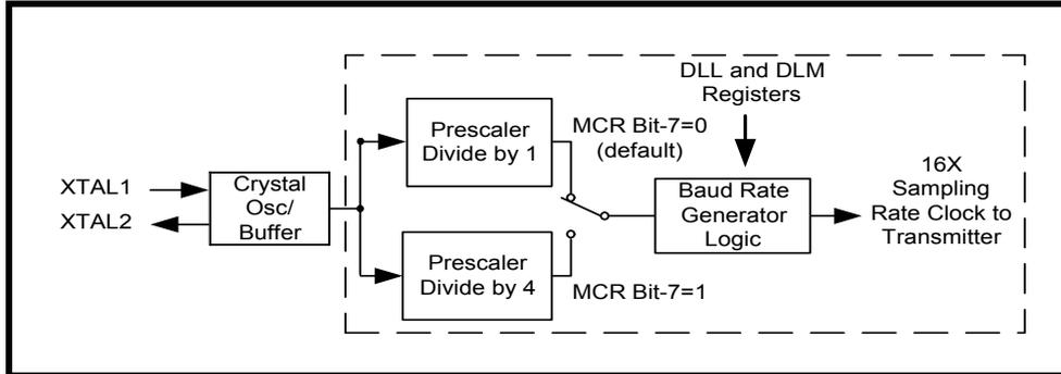
Table 6 shows the standard data rates available with a 14.7456 MHz crystal or external clock at 16X sampling rate. When using a non-standard frequency crystal or external clock, the divisor value can be calculated for DLL/DLM with the following equation.
