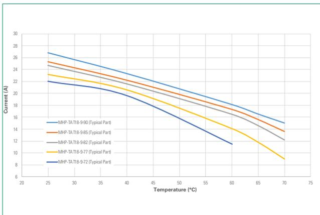
The current versus temperature curve was derived from placing test samples in an oven at 25°C, 40°C, 60°C, 65°C, and 70°C, increasing current flow through the sample at a rate of 0.1A/minute and recording the current value when the sample trips.
